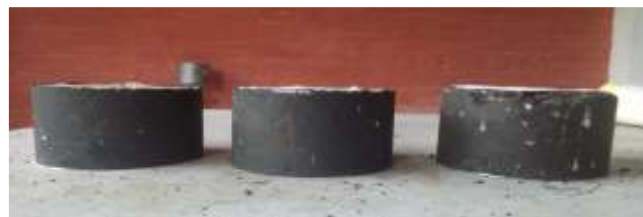
Fig. 7 Specimens containing 7% fly ash with varying bitumen content, 7%, 6.5% and 6% bitumen content
