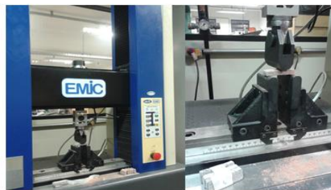
Fig. 6. Bending test in test specimen
