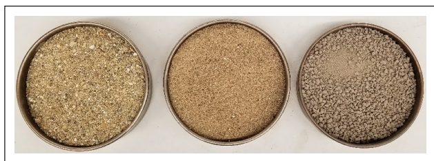
Figure 1. Leftmost pan shows natural sand, middle pan shows DS#1 and rightmost pan shows DS#2.
