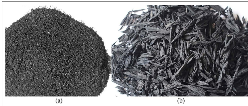
Figure 2. High-resolution photos of (a) crumb rubber and (b) tire chips.
