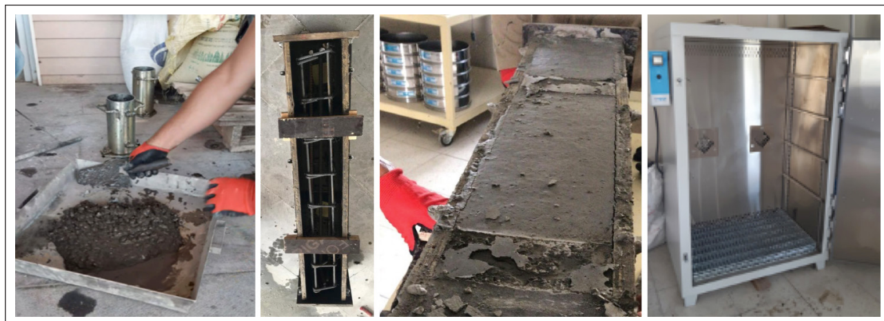
Figure 2. Placing and curing concrete in molds.
