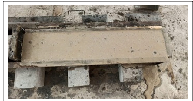
Figure 2. Mould with casted beam specimen.
