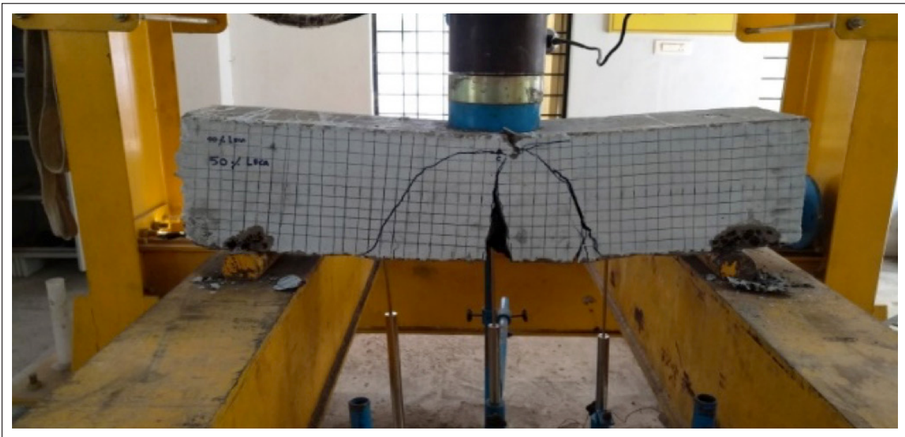
Figure 12. Crack pattern of beam LECA 25.
