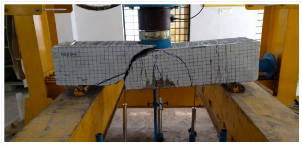
Figure 11. Crack pattern of beam LECA 20.
