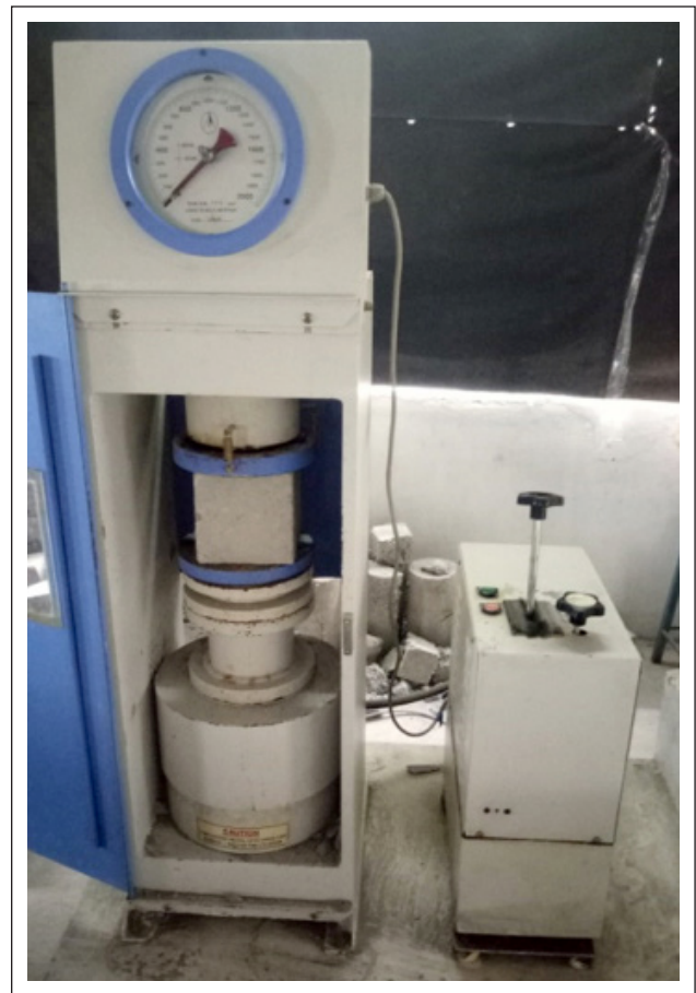
Figure 5. Experimental photograph of compressive strength test.
