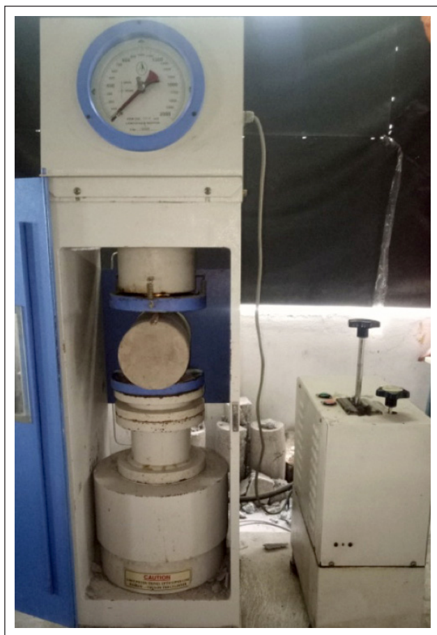
Figure 6. Experimental photograph of Split tensile strength test.
