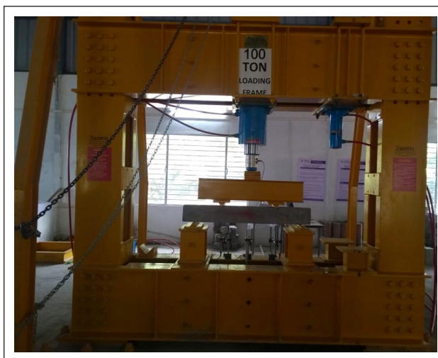
Figure 7. Experimental photograph of Flexural strength test.
