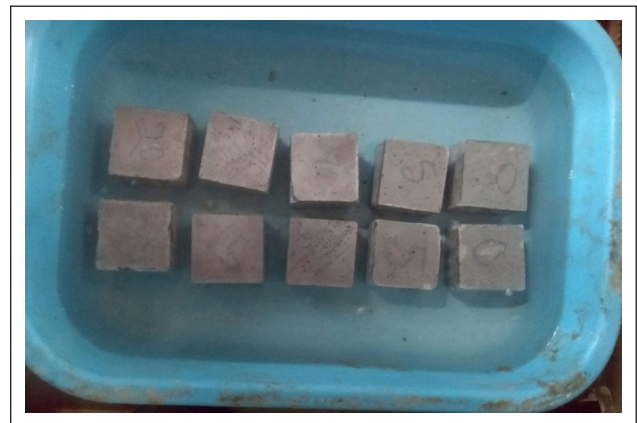
Figure 5. Water absorption test setup.
