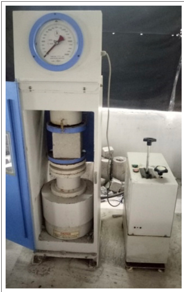
Figure 3. Compressive strength setup.
