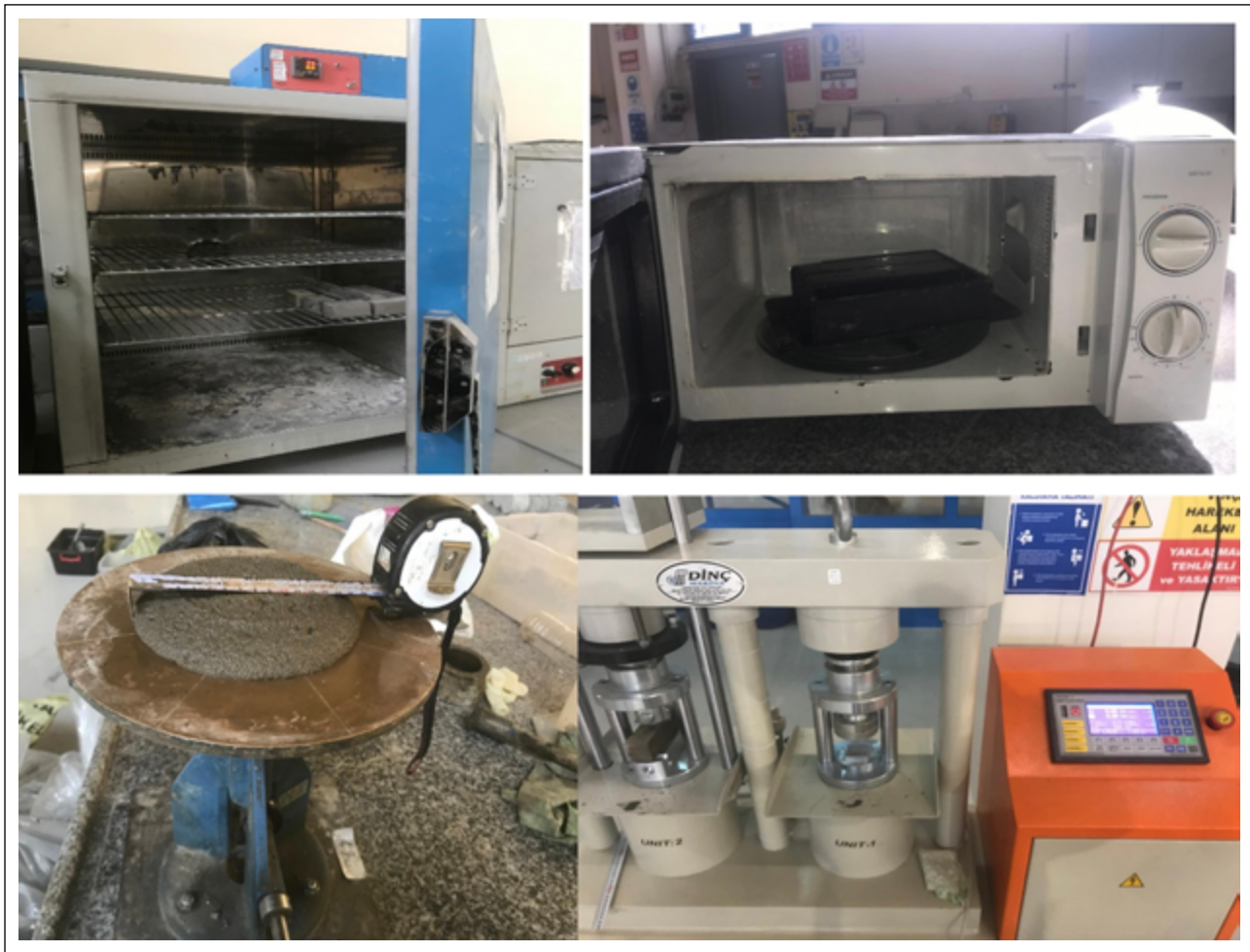
Figure 1. Curing setup and testing of GMs.
