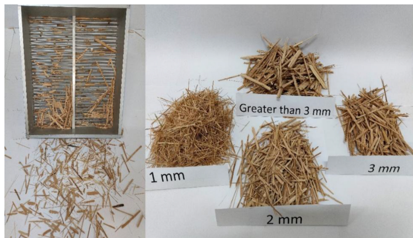
Fig. 4. Sorting wood chips according to their thickness using bar sieves.
