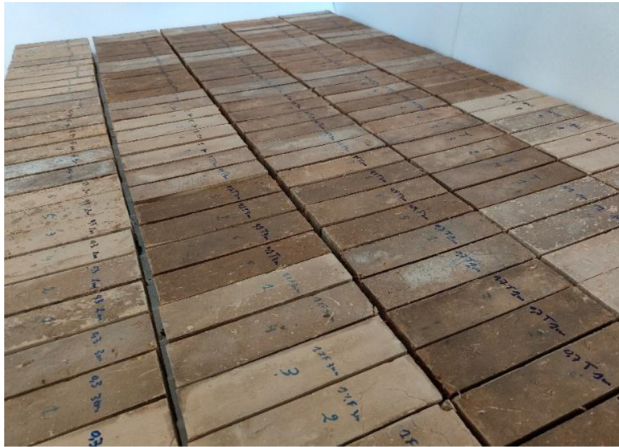
Fig. 5. The CEBs dry after the plastic cover is removed.
