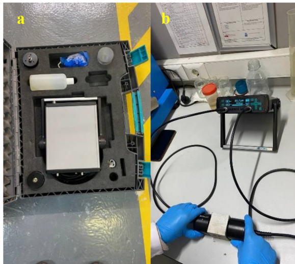
Fig. 5. (a) UPV device and (b) UPV experiment conducted on a cubic sample.
