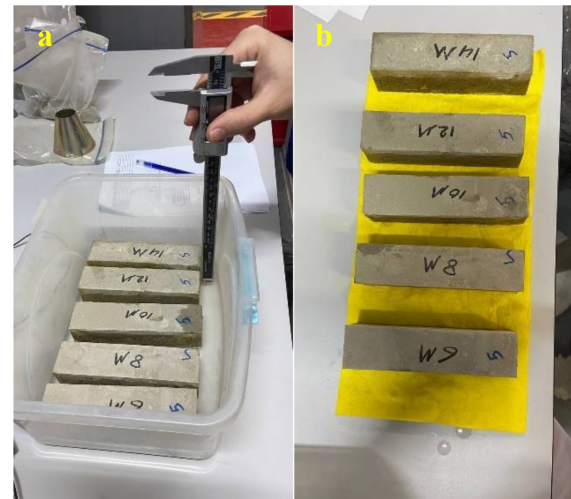
Fig. 6. Water absorption experiment: (a) before and (b) after extracting the samples from the container.
