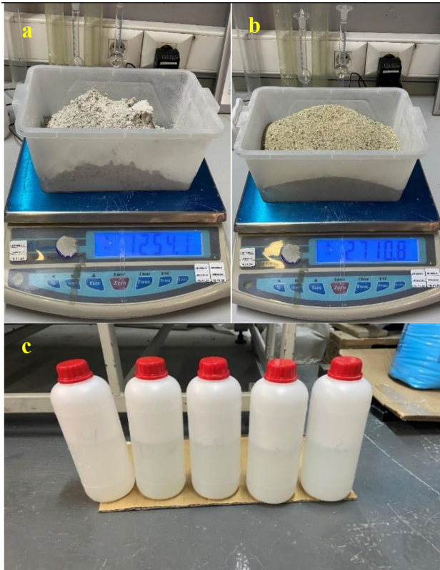
Fig. 1. The constituents that compose geopolymer mortars: (a) GGBS, (b) sand, and (c) NaOH solutions.
