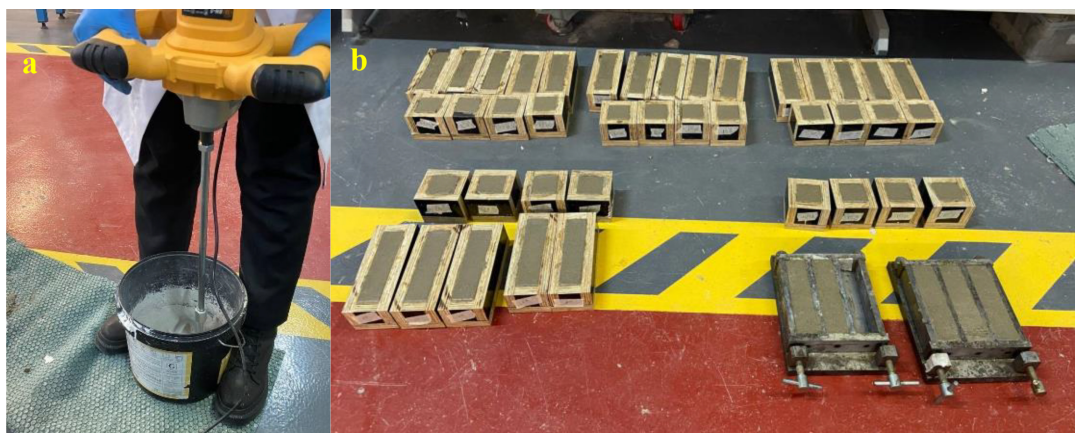
Fig. 2. Geopolymer mortar: (a) during the mixing process and (b) after pouring into the molds.
