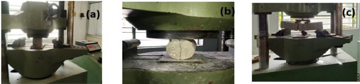
Fig. 6. Hardened test of UTM mixes: (a) CPS, (b) STS, and (c) FTS.
