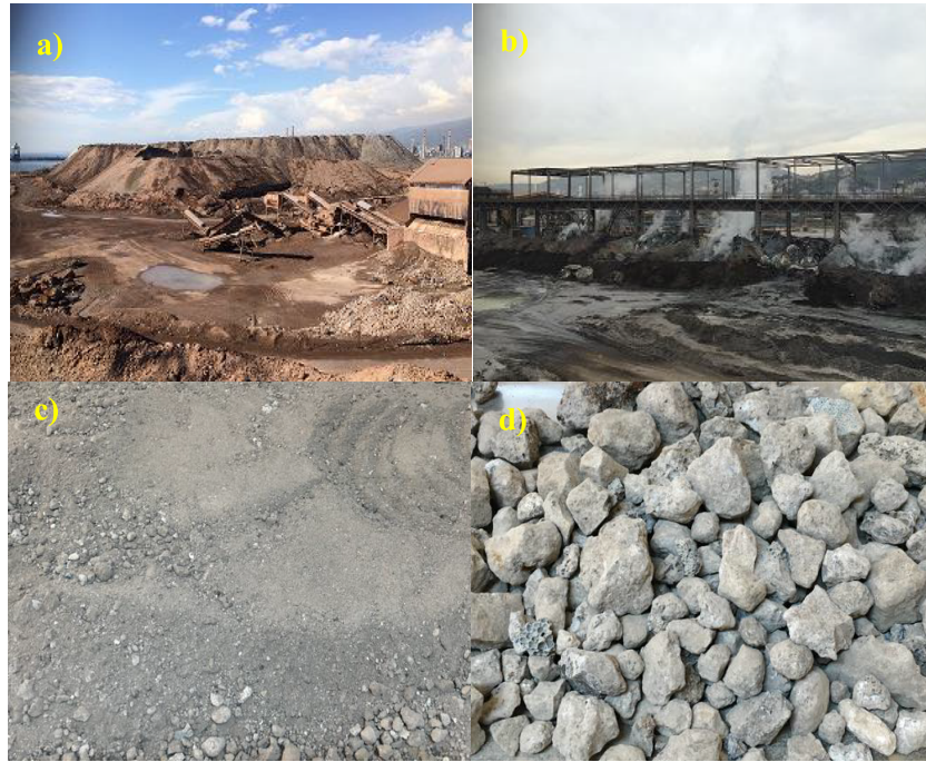
Fig. 1. (a) Stockpile of BOFS; (b) Cooling process; (c) Fine BOFS; (d) Coarse BOFS.
