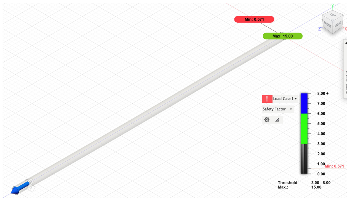
Fig. 7. No chances of failure at 23 KN (corresponding to a SF of 3).
