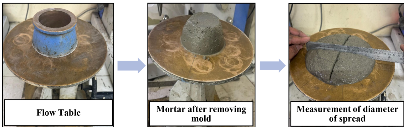
Fig. 6. Assessment of flow through the flow table.
