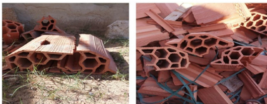
Fig. 9. Damaged hollow clay floor blocks.
