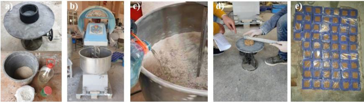
Fig. 3. Main process of slag based geopolymer mortar production: a) flow table apparatus and materials, b) mixer, c) mixing process, d) flow table test, e) moulded geopolymer specimens.
