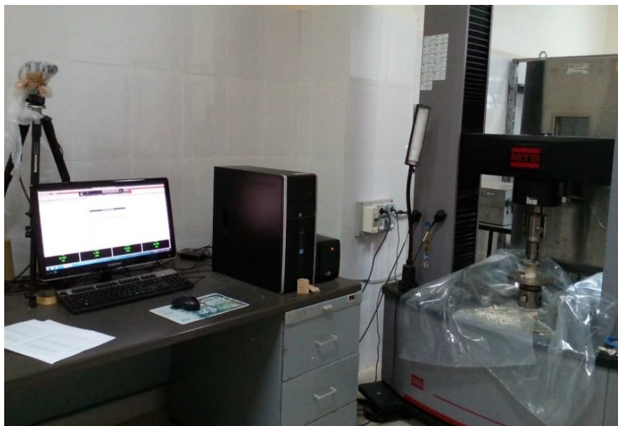
Fig. 6. MTS machine used for the compressive test of the historic mortar.
