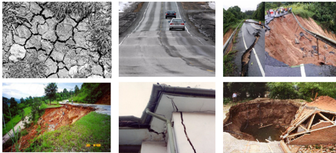
Fig. 1. Wet soil failure in different geotechnical forms: a.) Typical expansive soil [24] b.) Heaving of flexible pavement caused by expansive soils [25] c.) Highway slope failure on Khao Sok Mountain triggered by intense rainfall [26] d.) Weak plane failure along a section of the Mae Moh Dam access road [27] e.) Structural damage at the corner of a house resulting from soil heave [28] f.) Building damaged by a sinkhole collapse on April 23, 1997, above Permian gypsum in Ripon, NE England [29].
