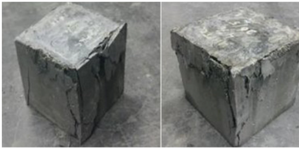
Fig. 10(a). Failure patterns of test specimens after compressive strength testing: Cube specimens showing typical vertical cracking and crushing at the edges.
