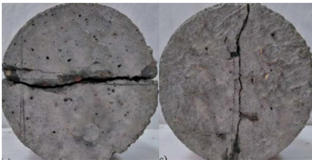
Fig. 10(b). Failure patterns of test specimens under axial compression: Cylindrical specimens exhibiting longitudinal splitting and shear-type failure.
