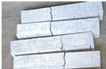
Fig. 10(c). Failure patterns of test specimens under flexural loading: Prism specimens exhibiting a single dominant vertical crack.
