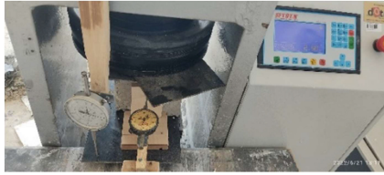
Fig. 3. Compressive strength test and longitudinal-transverse strain measurement.
