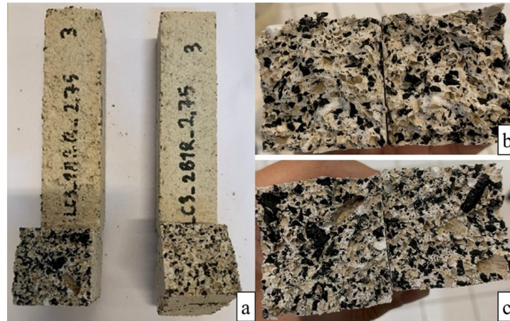
Fig. 3. The samples produced and their sections: a) LC-2R1B8-2.75 (left) and LC-2B1R8-2.75 (right), b) LC-2B1R8-2.75, c) LC-2R1B8-2.75.
