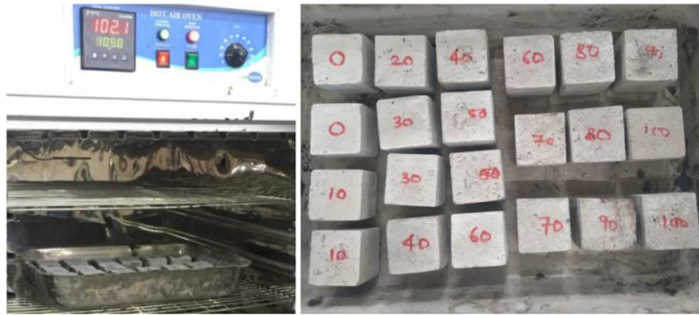
Fig. 4. Oven dried sample for water absorption test and density determination.
