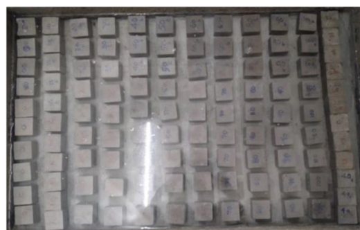
Fig. 10. Curing of BFS based mortar specimens.
