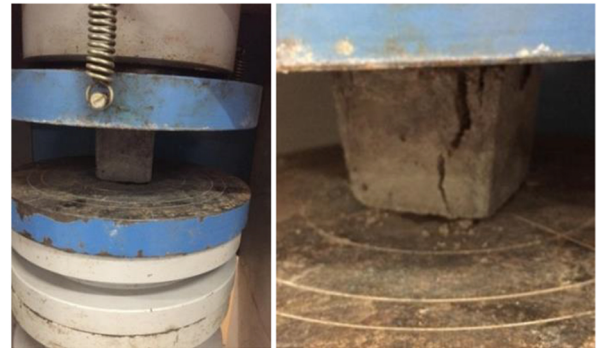
Fig. 5. Compressive strength test of BFS based mortar.
