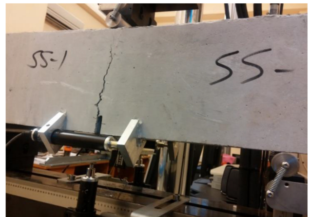
Fig. 4. CMOD controlled flexural loading.
