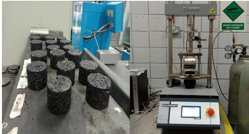
Fig. 3. (a) Marshall samples and (b) Marshall testing machine.
