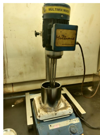
Fig. 2. High-shear multimix mixer used for blending modified asphalt binders.
