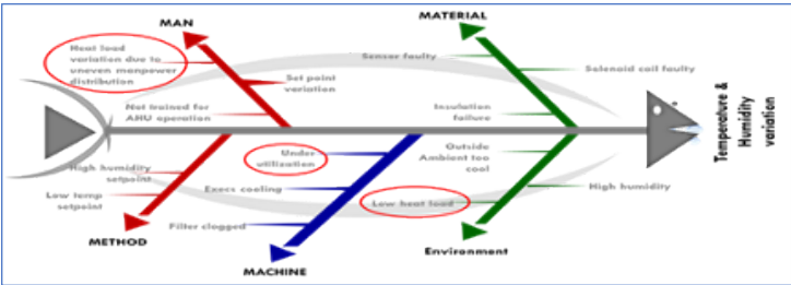
Figure 5. Ishikawa diagram done by the primary author as part of internal root cause identification
