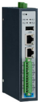
Figure 12. Edge Device used in the AI model used for Heat & humidity Calculation
