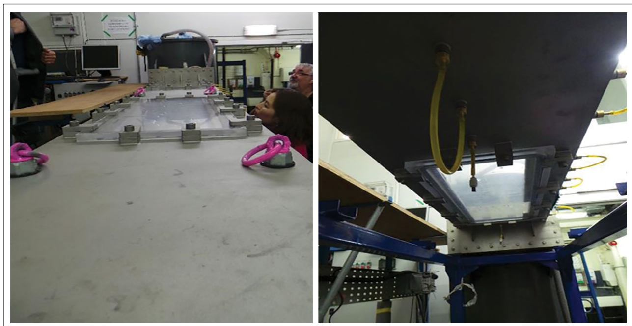
Figure 8. Two parallel smooth test panels (Surface A and its replicate) in place, top panel (L); bottom panel (R).
