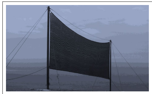
Figure 1. Fog harvesting mesh in the large scale (LFC) (Holmes et al., 2014).
